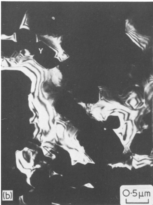
Figure 8 Transmission electron micrographs from the centre of the REFEL rod (SC8 R) showing (a) the bimodal SiC grain structure in bright field; (b) a dark-field image from the silicon matrix around the fine material and (c) a dark-field image taken using a reflection from the fine SiC material. The grains in (c) correspond to the location Y in (b) prior to tilting to the new diffracting condition.
